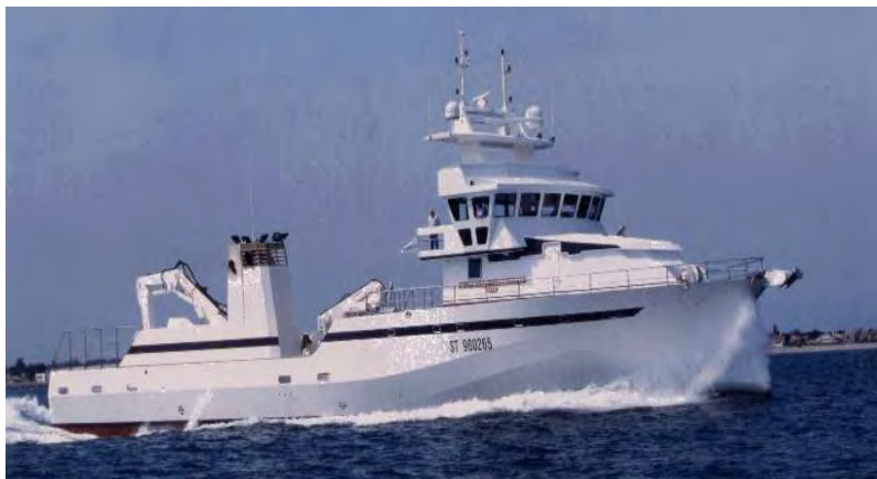
Picture 003.- Mediterranean type French PS tuna fishing vessel “Jean Marie Christian VII” built by CN Martinez SARL. Bureau MAURIC, Length: 40m, Beam: 10 m, Max. draught: 3,70 m, Speed: 17 knots, building: glass/resin composite, Holds capacity: 244 m 3 , G.O: 70 m 3 . (Picture Courtesy by: Architecte Bureau d'Etude Mauric-Marseille)
