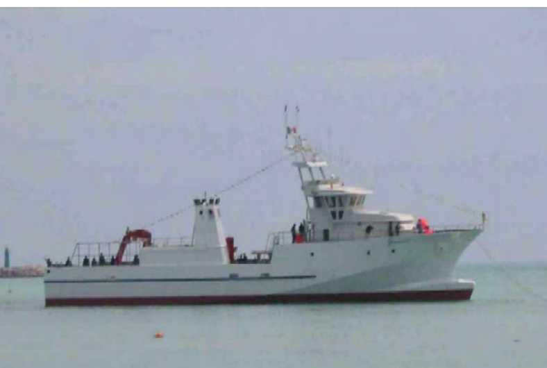
Picture 002.- Mediterranean type Italian PS tuna fishing vessel “Genevieve” built by CN Ortona Navi. Bureau MAURIC (Length: 42m, Beam: 9m, Max. draught: 3,60m, Speed: 17 knots, building: Steel hull, Alu. Superstructures, Holds capacity: 175m 3 & 58 m 3 ) (Picture Courtesy by: Architecte Bureau d'Etude Mauric-Marseille)
