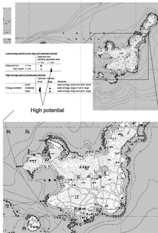
Fig. 5. Characterized points by physical environmental variables. In the inner bay and backreef points, points with less terrestrial influence are regarded as high potential areas. In the oceanward points, points with medium energy and low typhoon intensity are regarded as high potential areas. An example from Ishigaki island.
