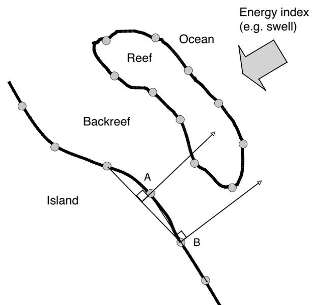
Fig. 4. Attribution of energy index. Vertical lines are set at each point, and if the lines are intercepted by other polygons, the point is regarded as protected, and null value is attributed (point A). Otherwise, energy index such as swell energy values are attributed (point B).
