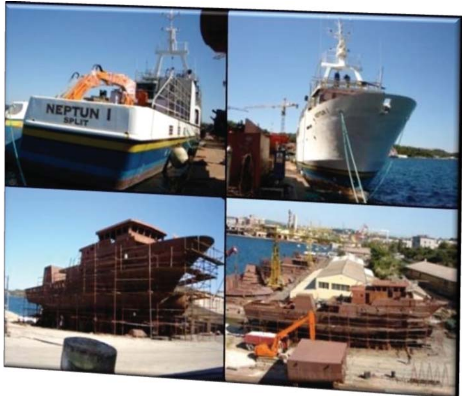
Figure 050: Croatian BFT purse seiners NEPTUNE I and NEPTUNE II under construction, seen at Pula Croatia on September 20 th 2007. They are two from a series of four BFT PS fishing vessels (LOA: 40.15 m, breadth: 8.65m, height: 4.20m, engine: 1600hp, speed: 14.5kn. builder: Tehnomont Pula shipyard) for Solin-Croatia-based BFT fishing operator Conex-Trade. Pictures ©©: Courtesy by: Siniša Jakši
